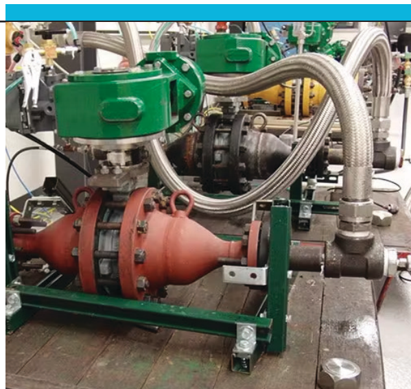
Fig. 1. Valves successfully being tested in a laboratory to PSA licensor specifications
